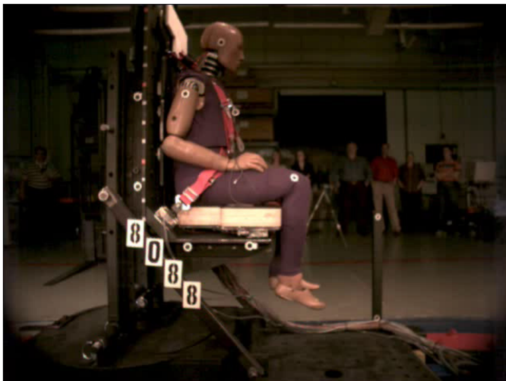
Figure 6. Dummy position in the x-direction with 10 g's impulse
