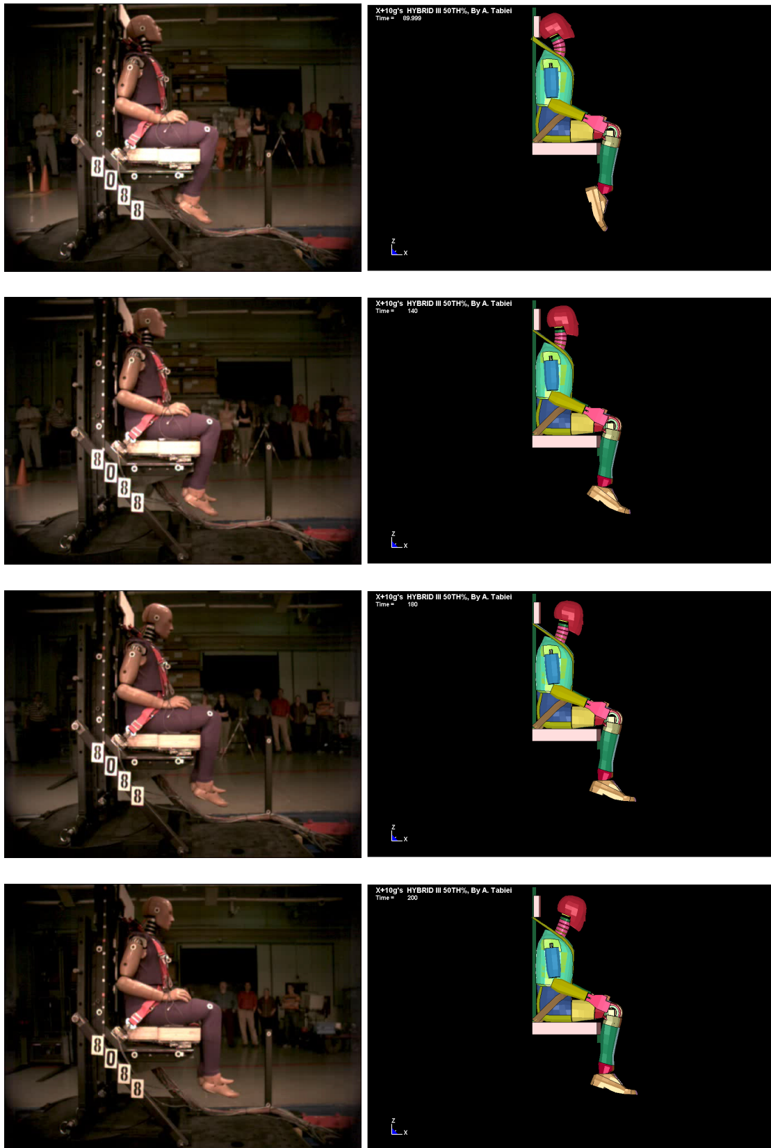
Figure 10. sled test in the x-direction at 10 g's pulse
