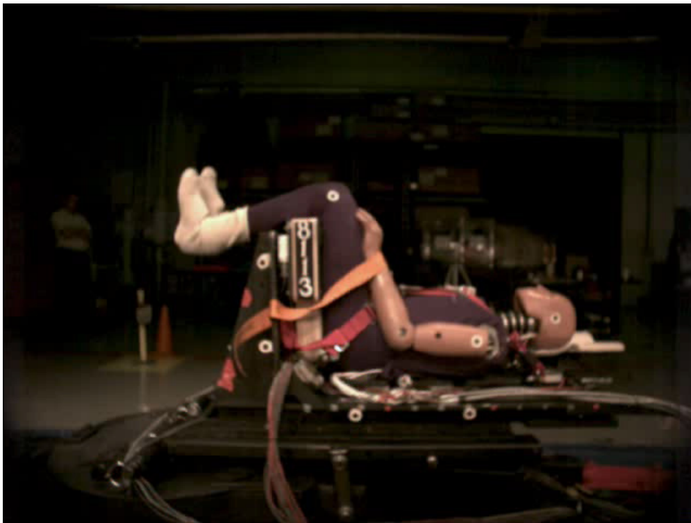
Figure 7. Dummy position in the z-direction with 20 g's impulse
