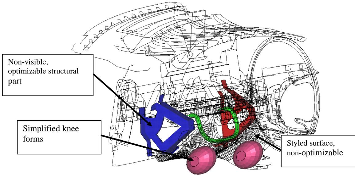
Figure 5: Instrument panel with knee bolster system (highlighted)
