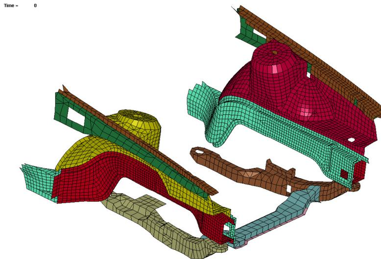
Figure 4: Parts containing thickness design variables
