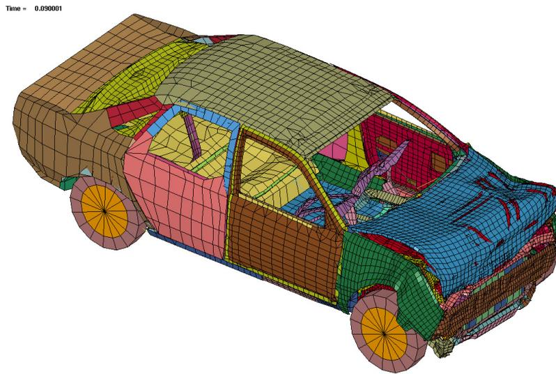
Figure 3: Deformed crash model of Taurus (90ms)
