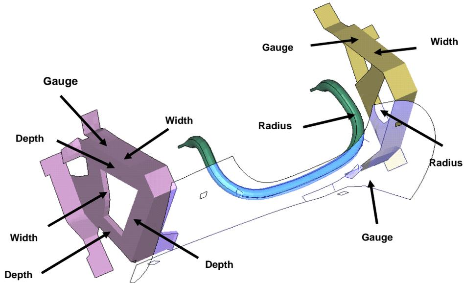
Figure 6: Eleven design variables of the knee bolster system
