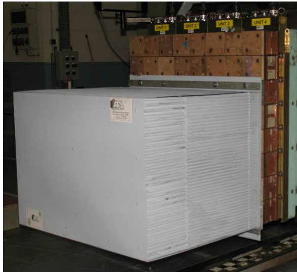
Figure 1. Progressive Deformable Barrier
