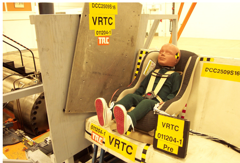
Figure 2. Experimental test dummy and CRS configuration.
