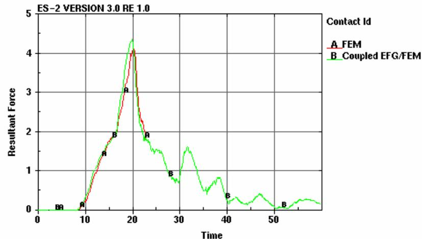
Figure 4 The Response Curve Comparison In The Dummy Component Test
