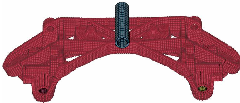
Figure 5(c) The Cradle Modeled By Meshfree Particles
