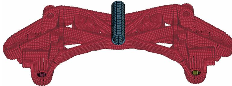
Figure 6 The Deformed Shape Of Cradle From The Coupled Analysis
