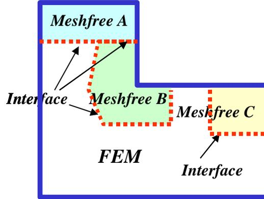
Figure 1 A two-dimensional model of coupled FEM/Mesh-free domain.
