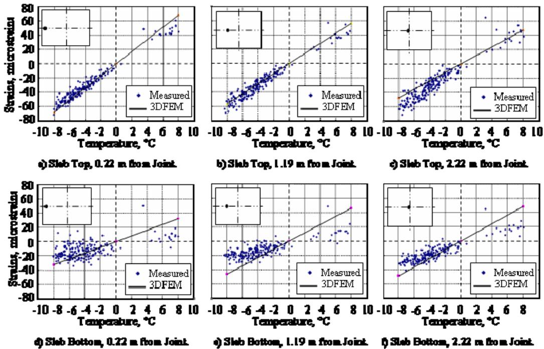
Figure 3. 3DFE-Calculated versus Measured Longitudinal Strains.
