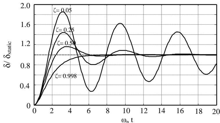
Figure 1. Displacement-Time Histories for Different Damping Ratios.
