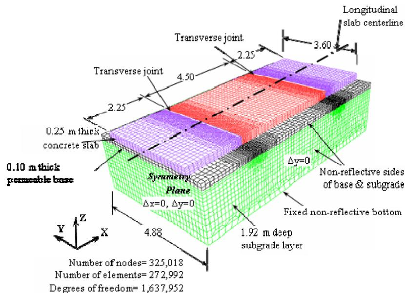
Figure 2 Finite element model of the concrete pavement
