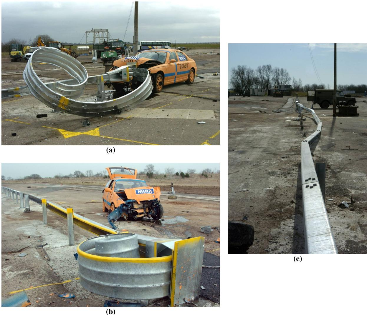
**FIGURE 8** After test images of the extruder terminal.
