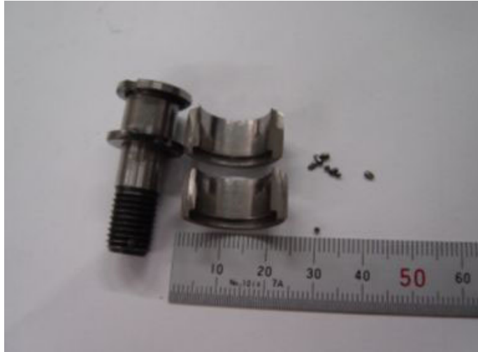
Figure 3. Worn out of needle bearing in stud-type roller
