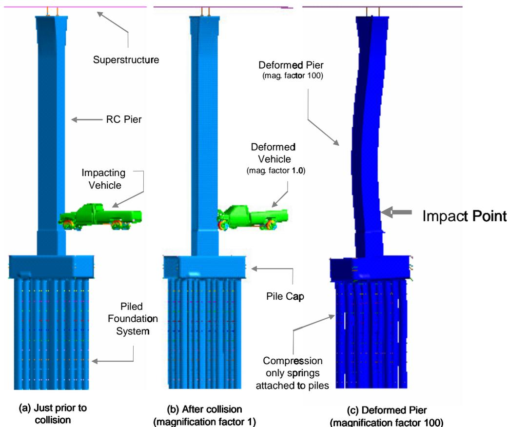
**Figure 3:** Model representing impact simulation between the Chevy truck and Pier I.
