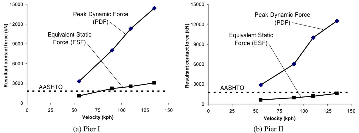
Figure 5: Impact force versus approach speed relationship for Chevy truck.
