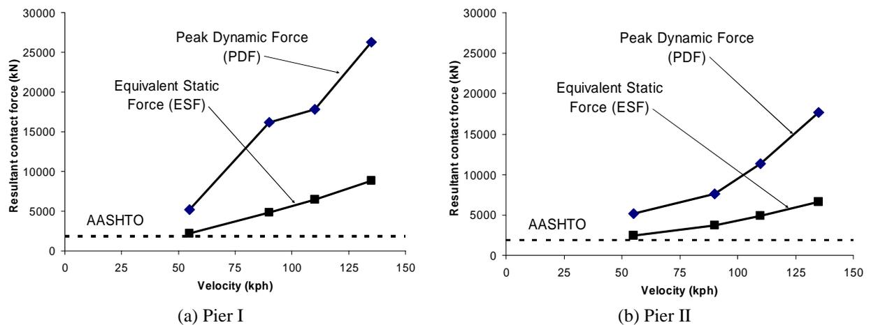
Figure 6: Impact force versus approach speed relationship for Ford truck.
