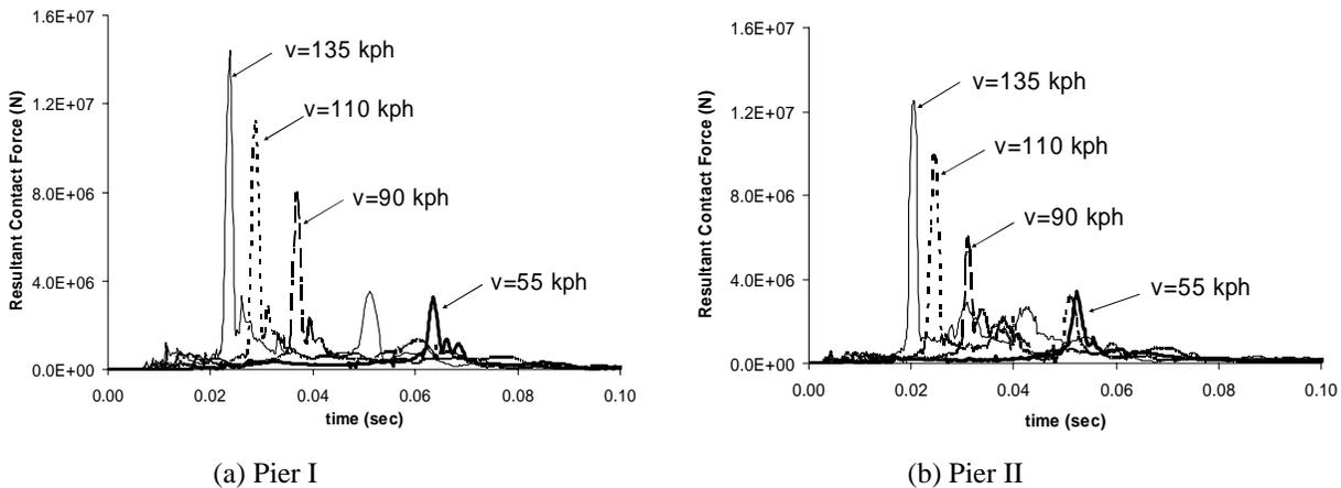
**Figure 4:** Impact force versus time for Chevy truck at various speeds approaching in transverse direction.
