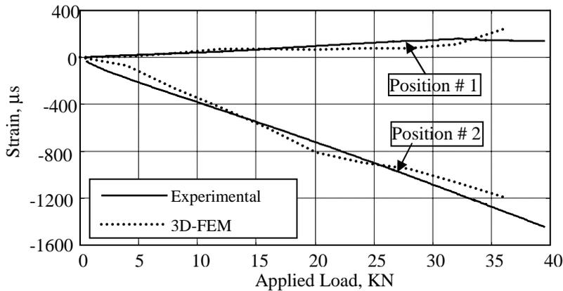
b. Measured and Calculated Strains.
