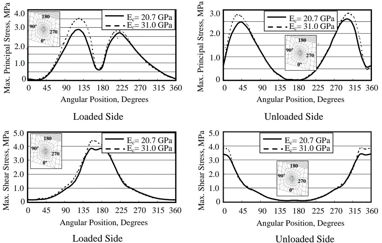
Figure 4 Distribution of Stresses Around the Dowel Bar Hole at Joint Edge.
