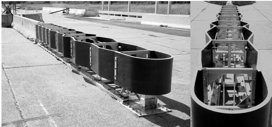
Figure 1. Hybrid Energy Absorbing Reusable Terminal (HEART) crash cushion.
