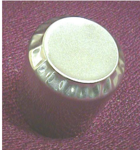
Figure 2. Photograph of redrawn beverage can showing profile wrinkles.
