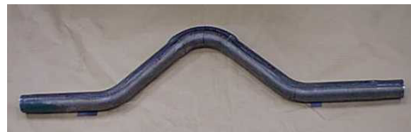
Figure 2. The bent and hydroformed “S” shape part
