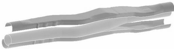
Figure 8. Finite element model for the pre-form and hydroforming
