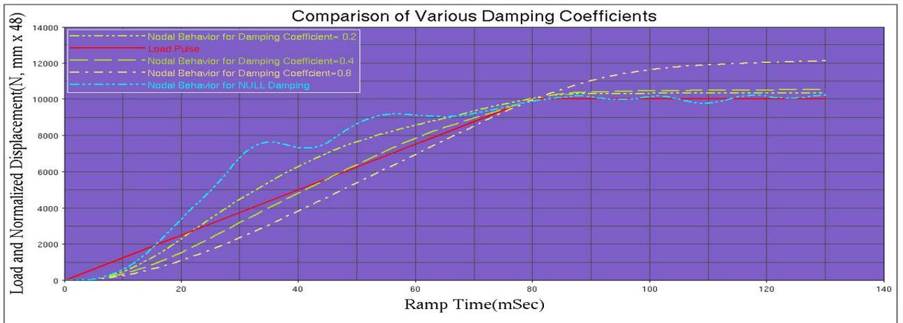
Figure 3: Effect of damping on the nodal displacement
