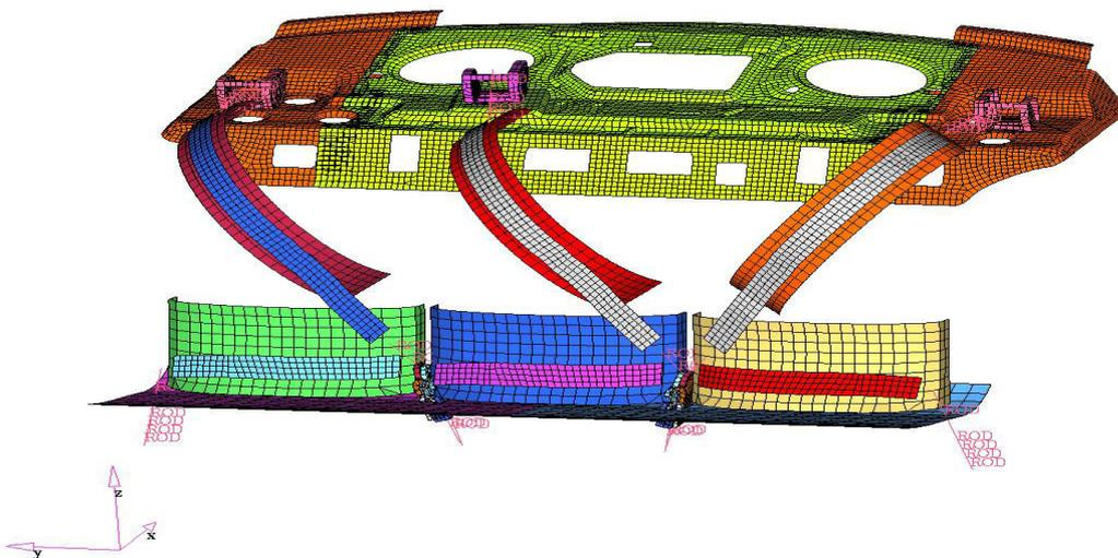
**Figure 1: Model details showing Pelvic and Torso Body Blocks**
