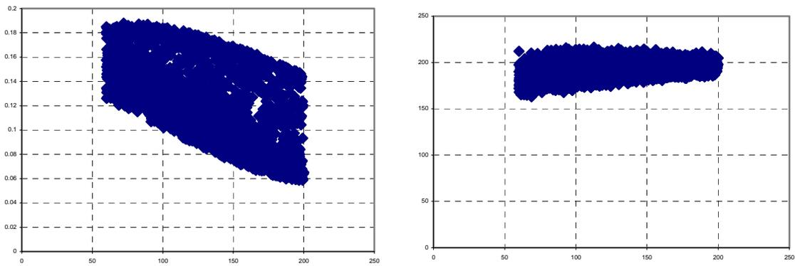
Plastic strain (left) and Average displacement (right) versus Ramp Time
