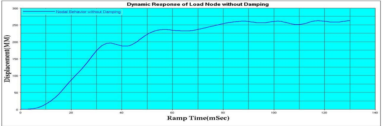
Figure 2: Dynamic Response of Load Node with no added damping
