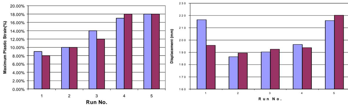
Figure 6: Comparison of LS-DYNA with Kriging predictions - Plastic strain (left) & Average Displacement (right)
