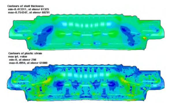
Figure 4. Option QUAD – Thickness (top) and plastic strain (bottom) contours.
