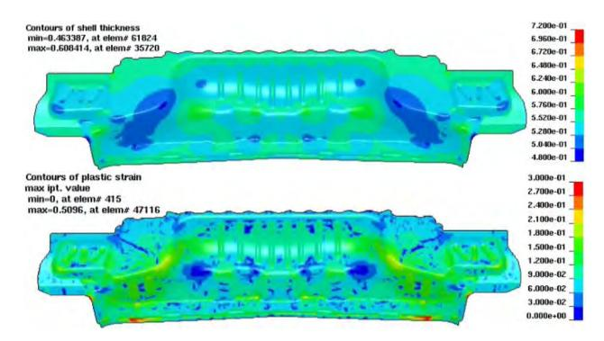
Figure 3. Option QUAD2 (default, recommended) – thickness (top) and plastic strain (bottom) contours.
