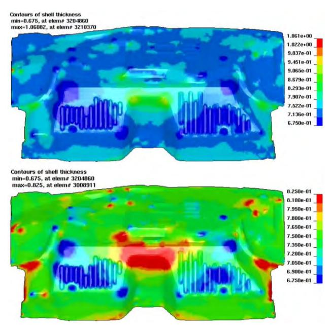
Figure 2. Maximum thickness scale factor (TSCLMAX) to limit the upperbound thickness values – top: no TSCLMAX; bottom: TSCLMAX=1.1); original thickness 0.75mm.
