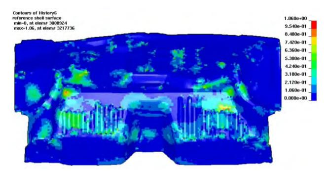
Figure 1. Damage accumulation in one-step simulation.
