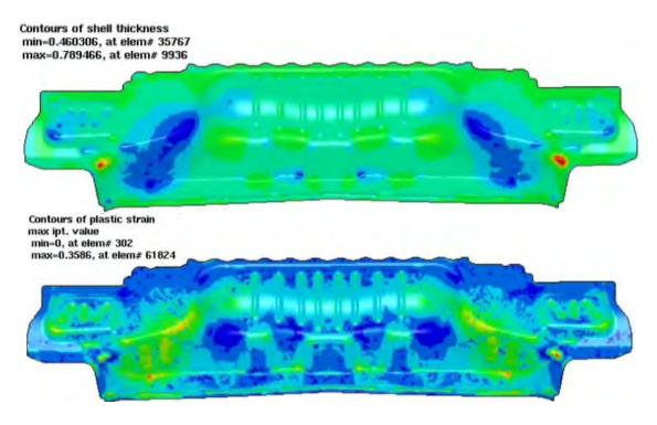
Figure 5. Option TRIA – Thickness (top) and plastic strain (bottom) contours.
