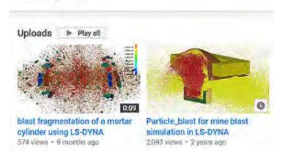
The Particle Blast Method (PBM) was employed to model the behavior of the detonation the bonded DEM was used to model the mortar cylinder, for more information, please refer to <a href="http://www.fragblast11.org/Media/Fragblast11/presentations/SESSION 10A 1150.pdf">http://www.fragblast11.org/Media/Fragblast11/presentations/SESSION 10A 1150.pdf</a>
