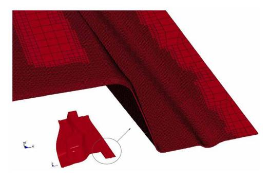
Figure 3. Adaptive mesh refinement of laminates (2005 NUMISHEET Crossmember).
