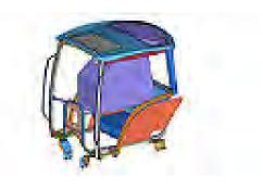
Fig. 2 CAD model of the tractor showing the protective structure FOPS
