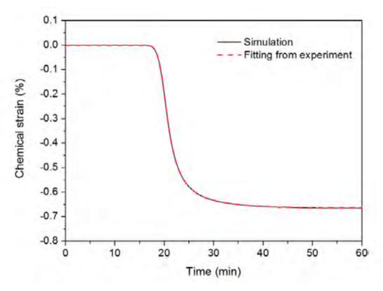
Figure 3 Chemical strain of MAT277 single element test
