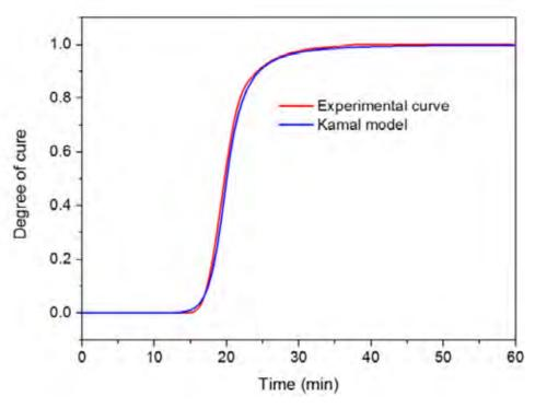
Figure 1 Curing degree of MAT277 single element test
