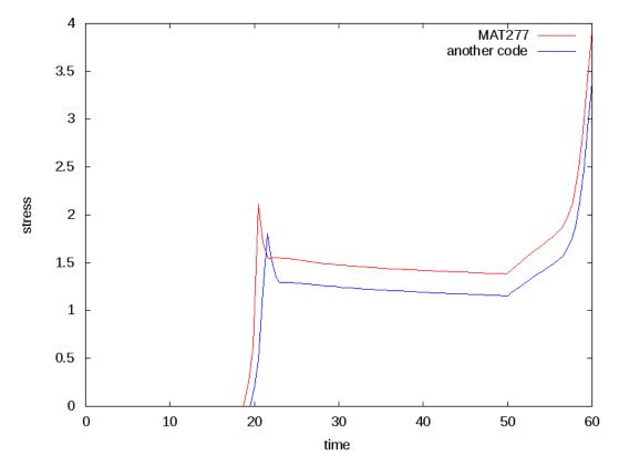
Figure 4 stress in xx direction of MAT277 single element test
