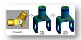
Figure 1: U-Joint Demonstration Model
