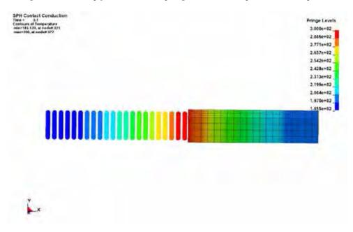
Fig 3. Temperature contour plot for thermal coupling between SPH part and Solid part
