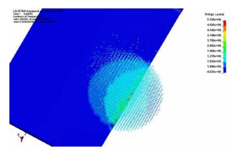
Fig 5. Temperature contour plot for HVI between Solid plate and SPH part with thermal coupling.
