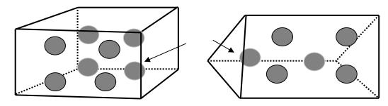
Fig 1. Transform Solid elements into SPH particles
