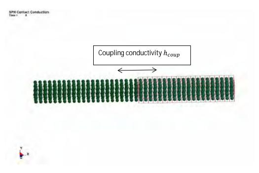
Fig 4. Hybrid element set up for thermal coupling between SPH part and Solid part
