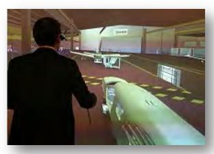
ESI's Immersive Virtual Prototyping solution allows Daher's engineers to immerse themselves inside their factory to set-up and fine-tune their aircraft final assembly lines.
