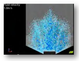
Motion of particles in the air flow using LS-DYNA Model No.404
