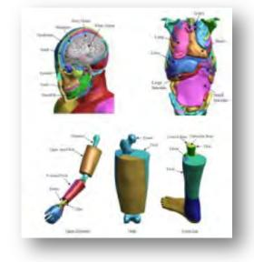
The Total Human Model for Safety, or THUMS<sup>®</sup>, is a joint development of Toyota Motor Corporation and Toyota Central R&D Unlike dummy models, which Labs. are simplified representation of humans, THUMS represents actual humans in detail, including the outer shape, but also bones, muscles, ligaments, tendons, and internal organs. Therefore, THUMS can be used in automotive crash simulations to identify safety problems and find their solutions.
