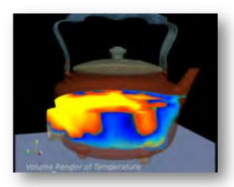
This simulation shows the powerful multiphysics capabilities of LS-DYNA. The CFD solver is coupled to the solid thermal solver and the Electromagnetism solver.
