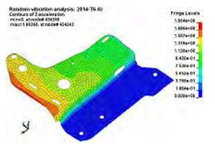
Figure 5. RMS of Z-acceleration
