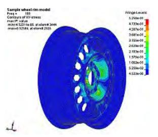
Figure 4. xy shear stress at frequency 100 Hz (magnitude)
