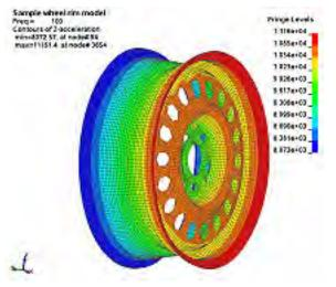
Figure 3. Z-acceleration at frequency 100 Hz (magnitude)
