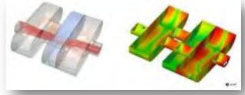
Simulation of an automotive muffler: CFD streamlines (left) and acoustic response (right)
