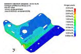
Figure 6. RMS of Von Mises stress
