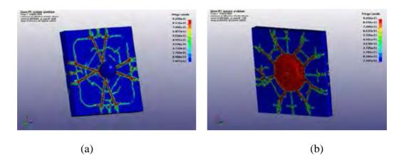
Fig. 15 The damage status by impaction, (a) the top surface; (b) the bottom surface
