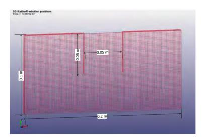
Fig .9 The dimension of specimen in Kalthoff-Winkler problem
