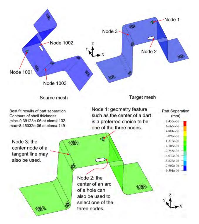
Best fit results - color contour of part separation plotted with "thickness" from the output file "Bestfit.out"
