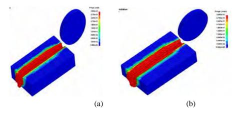
Figure 8. Final deformation in the SPG grooving simulation: (a) non-damage; and (b) damage.
