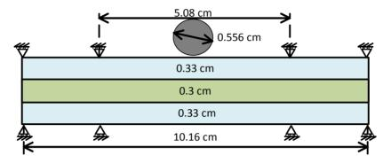
Fig. 12 The glass-PC-glass structure
