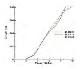
Fig. 10 The crack length history of Kalthoff-Winkler probem
