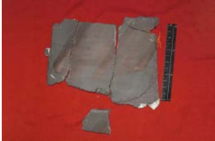
Figure 4. The major RCC fragments from the impact test.
