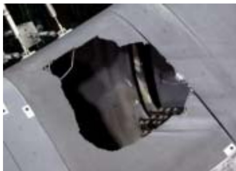
Figure 3. Close-up photograph of the damage to RCC panel 8.
