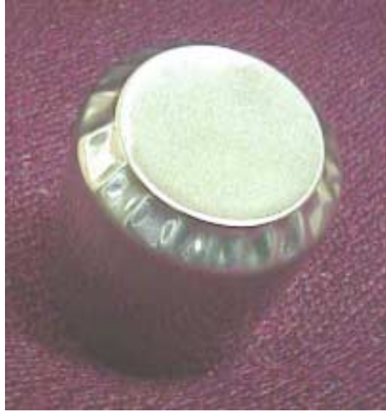
Figure 2. Photograph of redrawn beverage can showing profile wrinkles.
