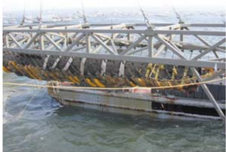
In the recovery of the Hunley, 32 slings attached to a steel frame supported the vessel's 65,000 pounds as a crane lifted the submarine to the surface.
