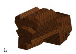
Fig 1. FEM mesh of a simplified auto engine model
