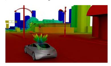
Simulation of an autonomous vehicle's lidar systems shows how accurately (red) or inaccurately (blue) certain objects are detected.
