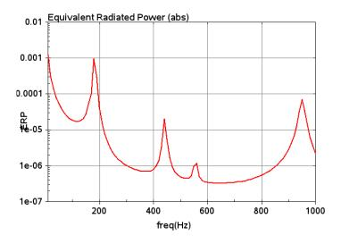
Fig 5. ERP absolute value (watt) vs. frequency
