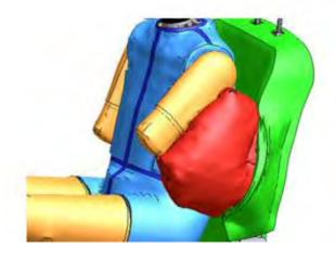
depends on the pattern through which it is folded. The risk of occupant injury during airbag deployment, the out-of-position problem, considerably affects the occupant's safety performance.
