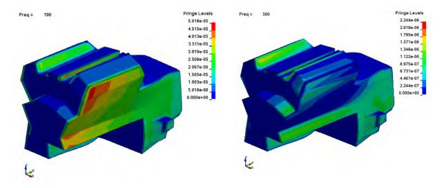
Fig 3. ERP density at frequency 100 Hz
