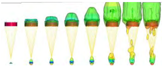
Finite Element Analysis of parachute deployment using porous membrane materials.
