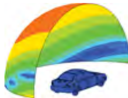
Vehicle radiated noise by BEM acoustic solver
