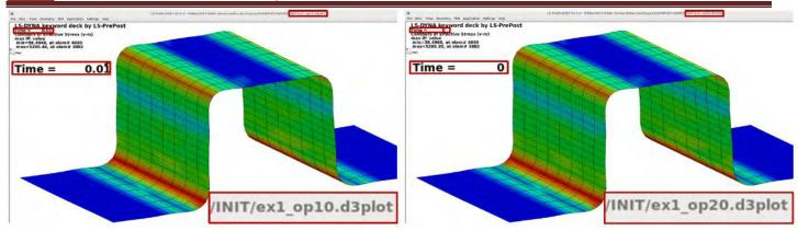
Fig.6: Von Mises Stress distribution: end of stage 1 (op10 - left) and beginning of stage 2 (op20 -right)
