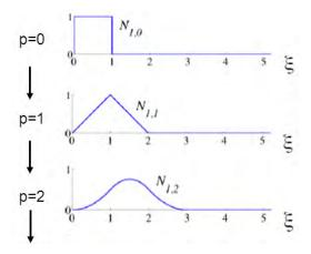
Fig.1: B-spline basis functions of order 0, 1 and 2 for uniform knot vector [3] The recursion formula is given by
