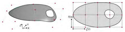
Fig.4: Trimmed NURBS surface with control points in physical space (left) and in parametric space (right)
