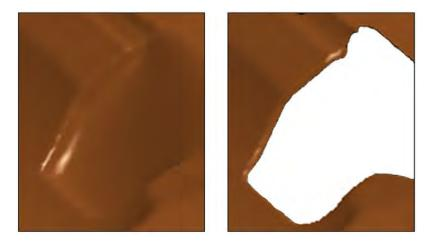
Fig. 7: A deformed shell NURBS patch before (left) and after trimming (right)
