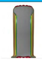
case1\_static\_flat\_P235\_55\_ R19.k In this case, the Tire is first inflated which is followed by compression of the Tire using prescribed motion of a
