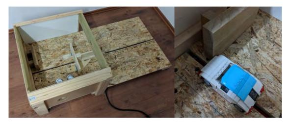
Figure 10: crash sled (left) and positioned car for 25% overlap frontal crash (right)
