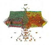
Bird striking CFRP laminate (SPH-Peridynamics)
