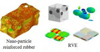
RVE analysis (Virtual material test module)
