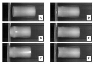
High speed camera images showing a plastic sabot impacting an aluminum plate at 114m/s, pin-jointed at it top. Sequence A-F, 0.1 ms between frames, highlighting sabot shock compression and residual plastic deformation.
