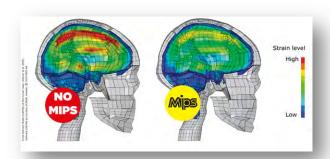
Finite Finite Element model (LS-DYNA) of the human head showing the maximum principal strain in the sagittal plane (Kleiven et al. 2003).
