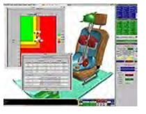
The Oasys HRMD Positioning T ool provides an interactive environment to set-up and analyse the positioning of the H-Point Machine in a s eat and to assess the head restraint scoring. All pre-simulation positioning of the HPM is completed automatically within Oasys PRIMER, and the output is a ready-to-run LS-DYNA model. Once the analysis is completed, Oasys PRIMER is used for interpretation of the results to report the H-point co-ordinates and back angle of the HPM.
