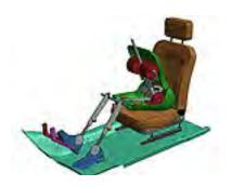
The Oasys HPM Positioning Tool provides an interactive environment to set-up and analyse the positioning of the H-Point Machine (HPM) in a seat.
