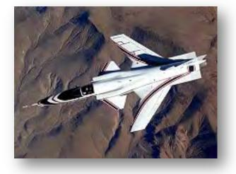
It looked like someone had installed the wings on backwards, and it was so unstable in flight that no pilot could fly it without the help of a computer, but the X-29A was a marvel in its day and provided research information useful for many aircraft designs still to come.
