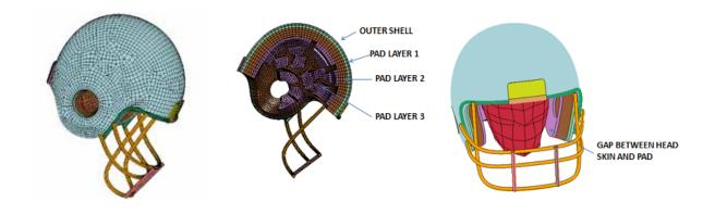
Fig. 3 Helmet Model and Energy Absorbing Pads.
