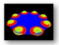
Plane detonation wave collision analysis using sph method
