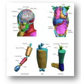
The Total Human Model for Safety, or THUMS®, is a joint development of Toyota Motor Corporation and Toyota Central R&D Unlike dummy models, which Labs. are simplified representation of humans, THUMS represents actual humans in detail, including the outer shape, but also bones, muscles, ligaments, tendons, and internal organs. Therefore, THUMS can be used in automotive crash simulations to identify safety problems and find their solutions.
