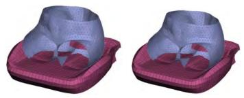
Figure 6. Before and after image of the dummy seat depenetration tool.
