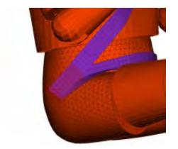
Figure 4. Belt with 2D \*ELEMENT\_SEATBELT definition
