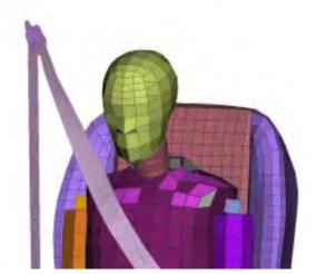
Figure 5. A seatbelt going through a 3D slipring
