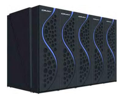
This system offers high performance and three times more energy efficiency per rack versus traditional air-cooled designs. It also produces 80% heat capture to the warm water for possible heat reuse.
