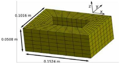
Figure 1 TEAM 4 Geometry and Mesh. Central hole:
