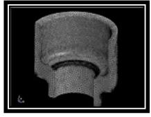
3D Forging Analysis using R-Adaptive Remesh with Local Refine
