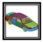
This example illustrates a realistic application of Multidisciplinary Design Optimization (MDO) and concerns the coupling of the crash performance of a full vehicle with torsional stiffness and mode frequency. LS-DYNA is used for explicit crash and implicit NVH and eigenvalue simulations.
