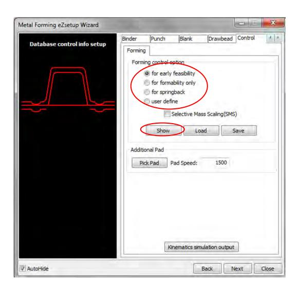
Figure 3. "Show" panel allows for changes to critical parameters
