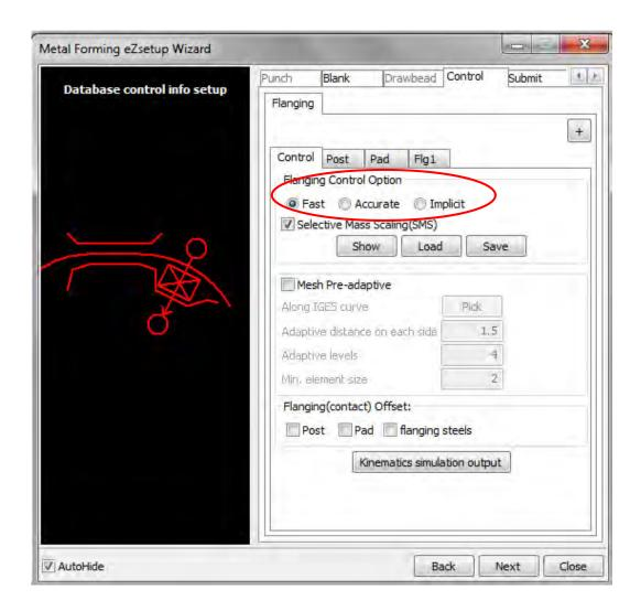
In the flanging process, there are also three computing levels to be selected, as shown in Figure 4. One of the levels is used for simulating flanging action in implicit static to reduce the inertia effect, especially in free-flanging case. Some of our users call this level as a 'high stiffness', or 'rigid' option, since dynamic responses of the unsupported area of the flanges are absent appearing to be more rigid.
