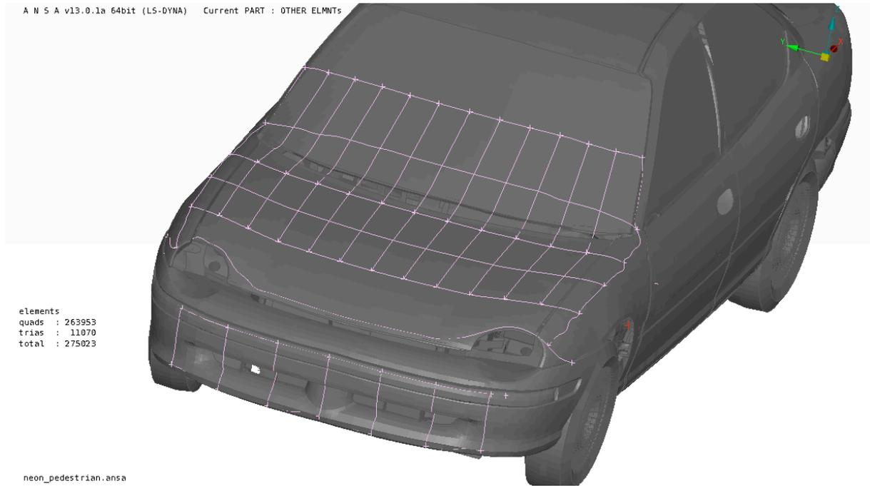
Figure 3. EuroNCAP reference lines automatically created
