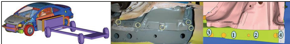
Figure 12: Side Impact simulation, post test with weld failure circled, post simulation showing the order of failure for each spot weld.
