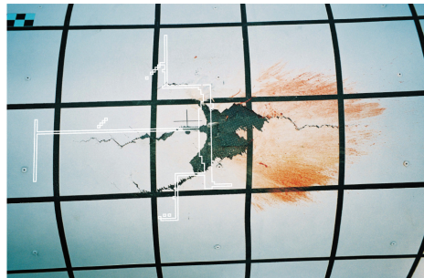
Figure 2: Comparison of test and simulation (white lines) results
