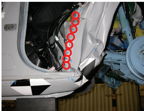
Fig.18 Ruptured spot welds at left rear door opening in the test
