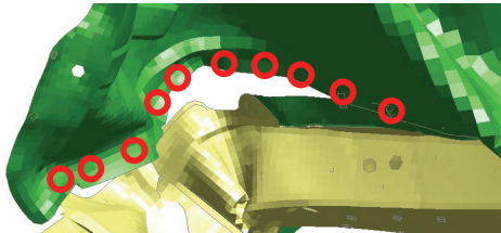
Fig.17 Ruptured spot welds at wheel housing in FE analysis
