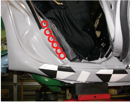
Fig.20 Ruptured spot welds at right rear door opening in the test
