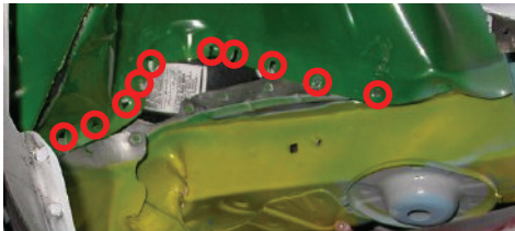
Fig.16 Ruptured spot welds at wheel housing in the test
