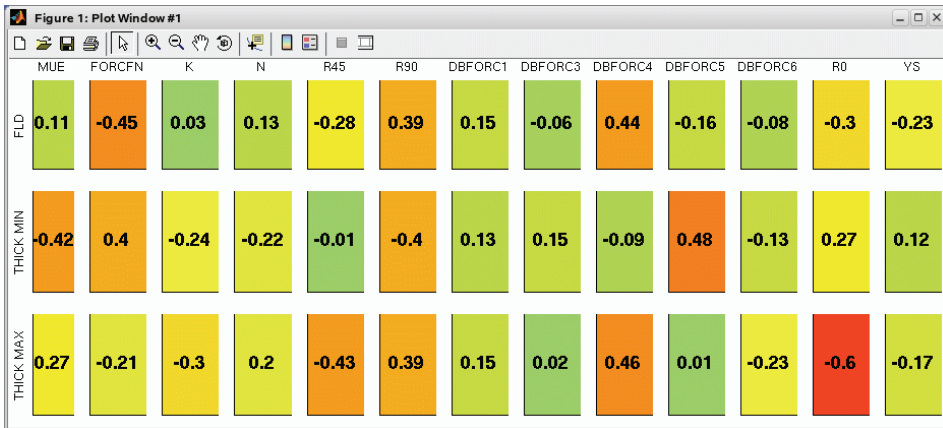
Fig. 10: Correlation of the uncertain parameters with respect to the responses minimum/maximum thickness and the distance to the FLC-Curve (noted by FLD)
