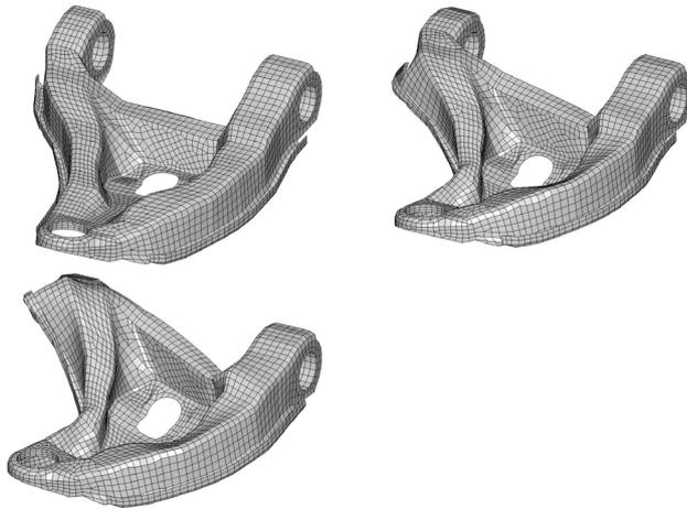
**Figure 5. Lower Control Arm Deformation Simulation**
