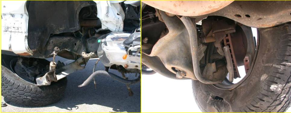
**Figure 4. Lower Control Arm Deformation That Occurs During Crash Testing**
