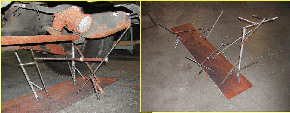
**Figure 6. Structure to Find Front Suspension Mounting Points**
