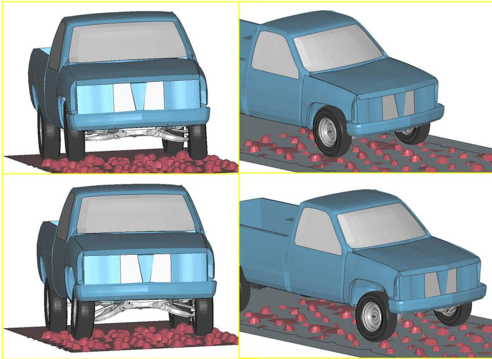
Figure 8. Rocky Ground Simulation Sequential Photos
