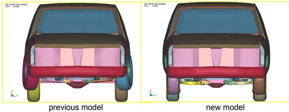
Figure 7. Improper Steering System Geometry Fixed
