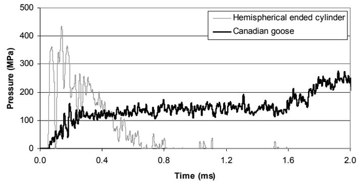
Figure 7 Stagnation pressure (centre of panel target) predicted for the impact of a multi-material bird model, compared to a hemi-spherical ended cylinder.
