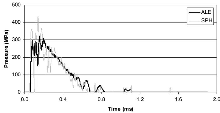
Figure 3 Stagnation pressure (centre of target) predicted for the impact of a hemi-spherical ended cylinder into a square flat panel.
