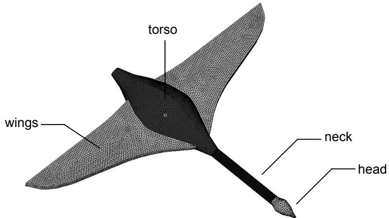
Figure 6 Schematic of the multi-material bird model used in the SPH simulation.
