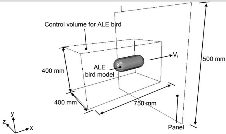
Figure 1 Schematic showing the bird-strike model for a square flat panel impact.
