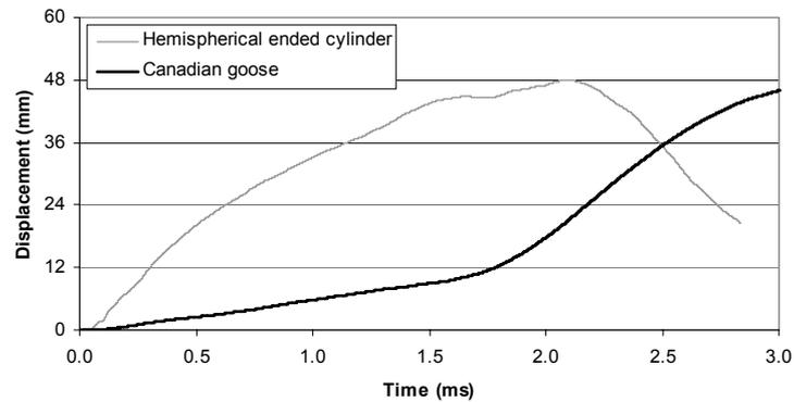
Figure 9 Resultant displacement (centre of panel target) predicted for the impact of a multi-material model, compared to the hemi-spherical ended cylinder.
