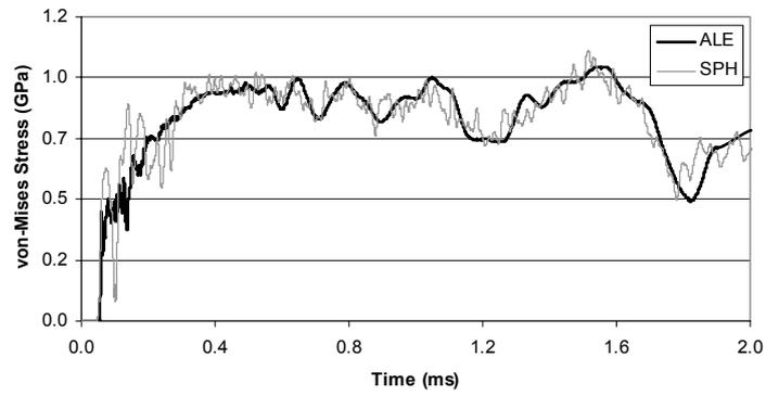
Figure 4 von-Mises stress (centre of target) predicted for the impact of a hemi-spherical ended cylinder into a square flat panel.
