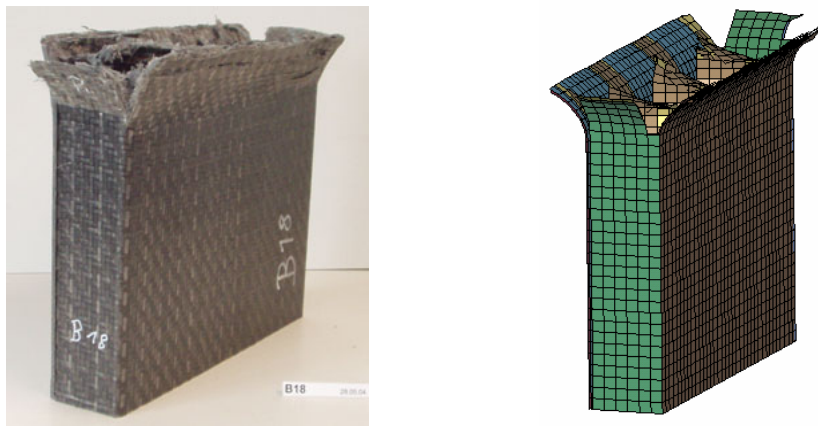
"Fig. 3.10: Comparison of deformation pattern experiment vs. simulation (Mat58) – perspective view"
