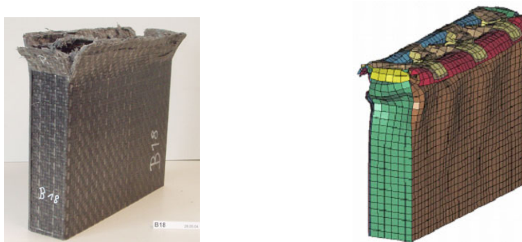
"Fig. 3.8: Comparison of deformation pattern experiment vs. simulation (Mat54) – perspective view"
