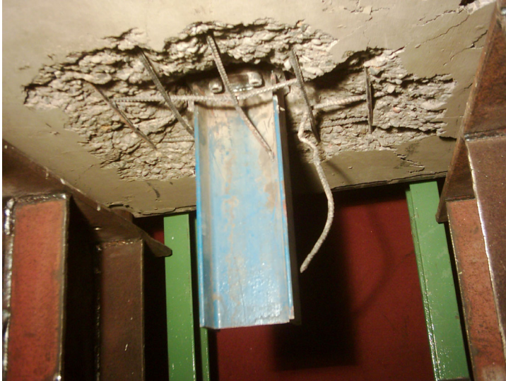
Figure 10 7.0m/s drop resulting in perforation
