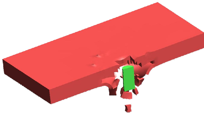
Figure 3 Solid projectile perforating slab (500kg object at 14.0m/s into 200mm RC slab without steel decking)
