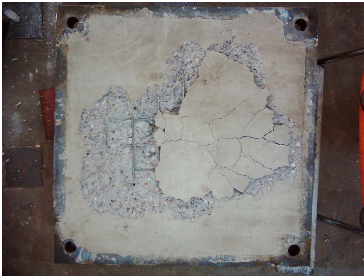
Figure 11 3.8m/s drop penetrating but not perforating
